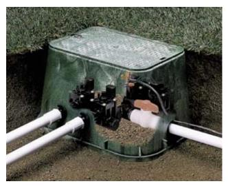
If the box is installed to high, protruding above the turf, it presents a physical hazard for turf care equipment and a potential trip and fall hazard for workers and pedestrians. A box installed below finish grade creates an unanticipated "hole" or low spot in a turf area. This affords an opportunity for turf to overgrow the edges of the box, further obscuring its' visibility. A box set too low, partially hidden by turf grass is a dangerous condition for maintenance worker and pedestrians.
